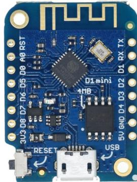
A mini wifi board with 4MB flash based on ESP-8266EX.
